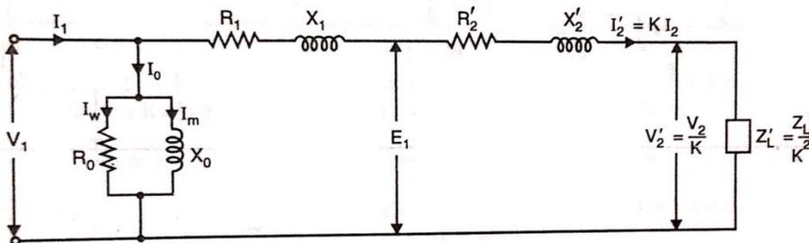
$V_1$  - Primary Input voltage
