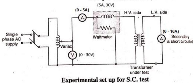
1½ Mark for SC test circuit diagram
