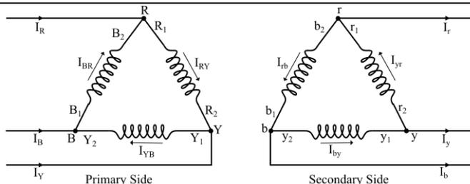
2 Marks for winding diagram
