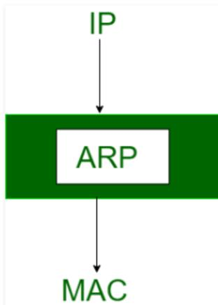
ARP finds the hardware address, also known as Media Access Control (MAC) address, of a host from its known IP address.
