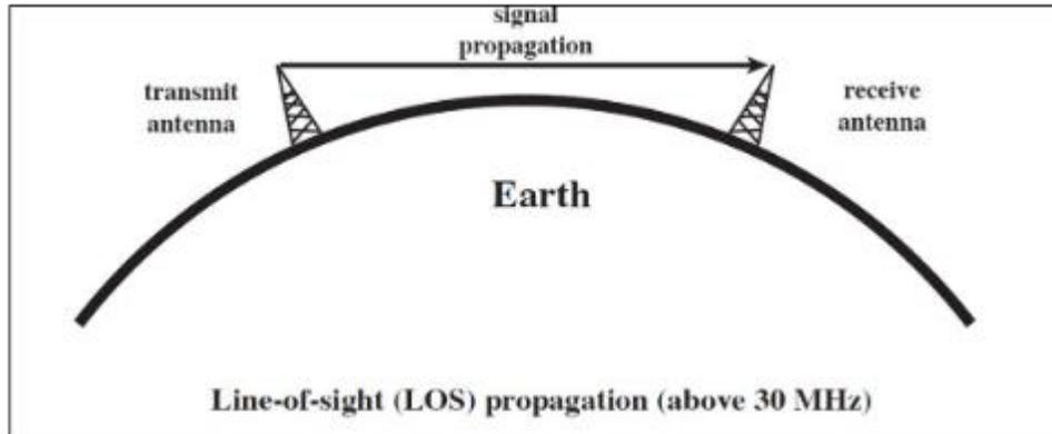
The figure depicts this mode of propagation very clearly. The line-of-sight propagation will not be smooth if there occurs any obstacle in its transmission path. As the signal can travel only to lesser distances in this mode, this transmission is used for infrared or microwave transmissions.
